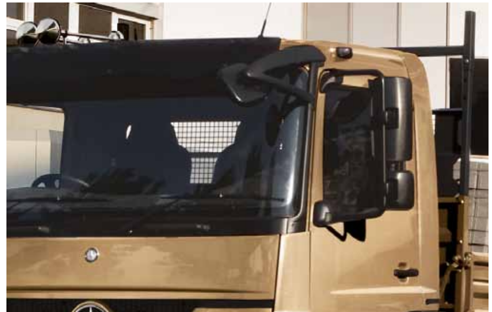
Fitted as standard, the large exterior mirrors can be heated so they do not mist or ice over or become prone to bedded-in dirt particles. The wide-angle rear-view mirror is mounted below the main mirror so as to provide better visibility. Furthermore, the new front bumper view mirror, reduces front blind spots and enhances safety.
