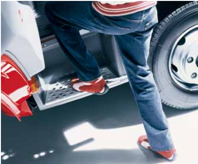
All aboard please: on some models, one step is enough, with a height of a mere 818 mm from road surface to cab floor. Drivers of Atego distribution trucks in the weight category up to 10.5 tonnes, who have to get in and out perhaps 30 or 40 times a day, are sure to appreciate this. On the Atego from 13 to 15 tonnes, two steps are enough
