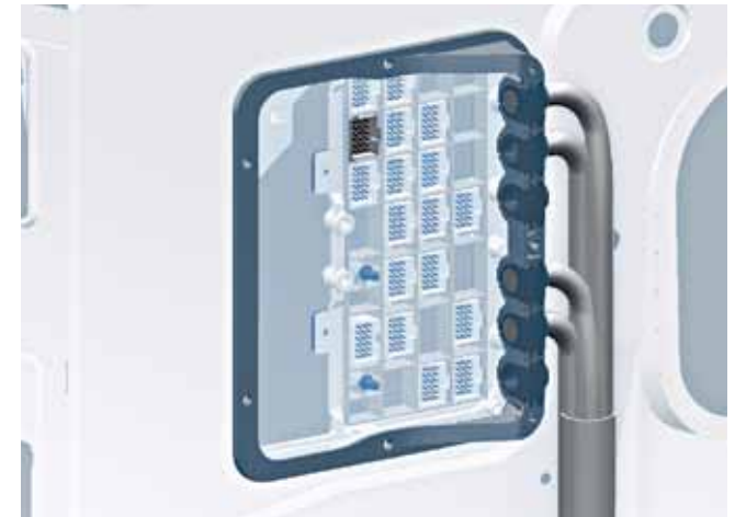
Less time-consuming, lower costs, improved reliability: the new body manufacturer interface, integrated centrally in the hatch below the cab's front-end flap, makes it easy to establish connections without the need for tiresome cable routing. Communication between the cab and body is simplified and body manufacturers gain easier access to the electrical systems
