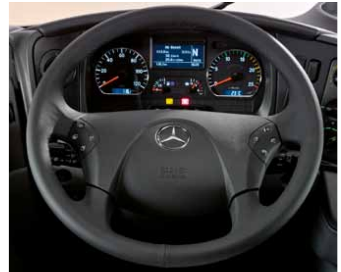
The new easy-grip steering wheel has a pneumatic adjustment mechanism: the height can be adjusted by 66 mm, whilst the angle can be set between 22 and 39, meaning that each driver can set the ideal position and get in and out of the cab easily
