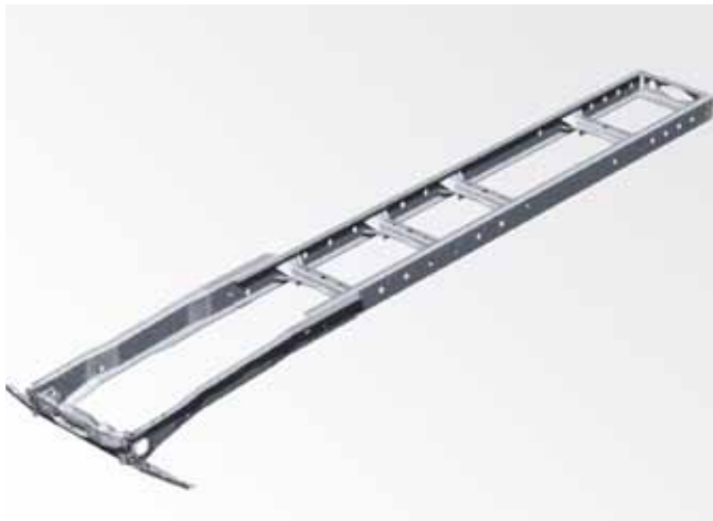
The frame's 50-mm hole pattern enables bodies and other units to be mounted both quickly and inexpensively. The fact that no extra drilling is required, avoids damage to the corrosion protection provided by the cathodic dip coating process
