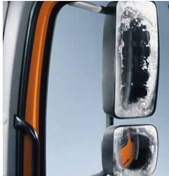
No misting over, no icing over and no burning-on of dirt particles, since the standard-fit electric heaters for the large exterior mirrors can be controlled manually. The wide-angle rear-view mirror is mounted below the main mirror so as to provide better rear visibility. New front bumper view mirror reduces blind spots and enhance safety.
