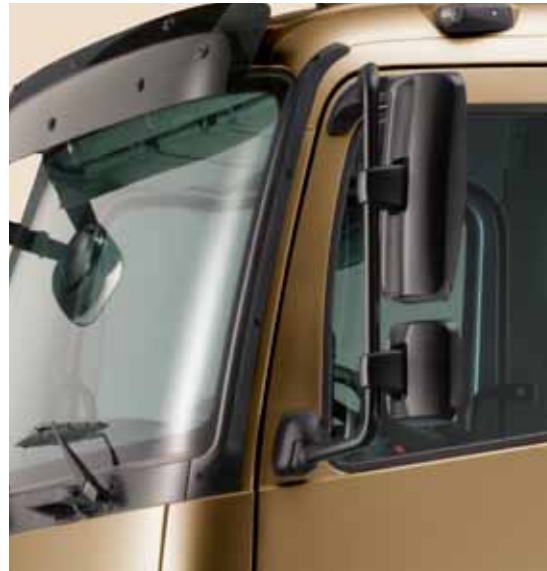
The wind deflectors on the A-pillar, exterior mirror fairings and corner panels to improve aerodynamics and reduce dirt build-up on the side door and side window.
