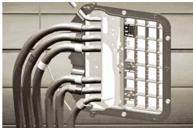
Simple connections without tiresome Cable routing: the new body manufacturer interface, integrated centrally in the Cab hatch, simplifies communication between the Cab and the body and affords the body manufacturer easier access to the electrical systems.
