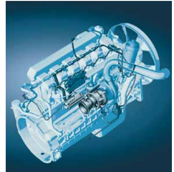
Axor trucks have the "Turbobrake" engine brake, a wear-free auxiliary brake which increases the boost pressure and, therefore, increases the engine braking effect to as much as 300 kW.
