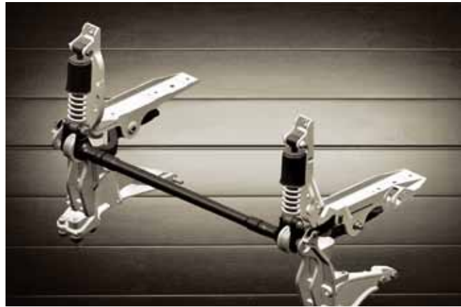
The new Cab mountings with additional longitudinal mounts and rubber mounts ensure better damping of shocks and vibrations caused by uneven road surfaces, for example.
