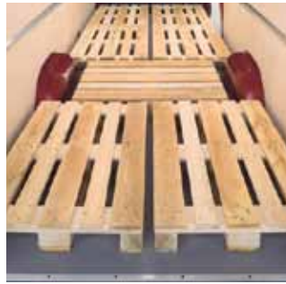
Up to 5 Euro pallets and full bulkhead (standard)
