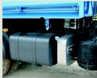
Remember the name BlueTec - it will be part of your future. Note the separate tanks for diesel and AdBlue (bottom left)
