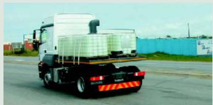
The local DaimlerChrysler testing facility in East London includes a chassis dyno but on-the-road driving tests with simulated loads are conducted around the Eastern Cape on a daily basis. This test centre has been incorporated into the international DaimlerChrysler development process.
