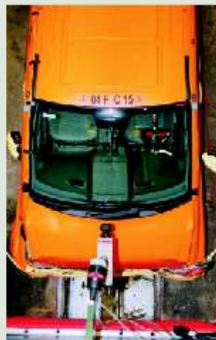
Actual crash tests are the final stamp of testing following computer simulations of passive safety features.
